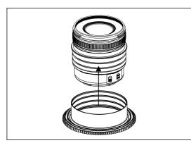
2. Insert the gear of C1018-Z on the plastic c-ring until it reaches the flange of the plastic c-ring.
